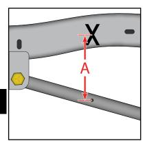
**Step 2.)** Mark a Dot on the moving suspension arm directly under the "X" from step 1, (This will be your target ball stud mounting point). With the vehicle at the top of its travel (aired all the way up), measure from your dot up to the center of your "X". We will call this distance "A".
