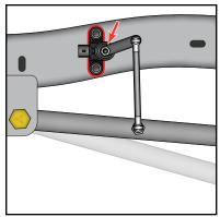
Step 8.) With the vehicle at the very bottom of the travel, hold the sensor at the same location traced on the frame in step 7. Either rotate the sensor slightly, or adjust the linkage so that there is about 1/4" of clearance between the upper plastic stop and the rotating arm. Visually note this amount.
