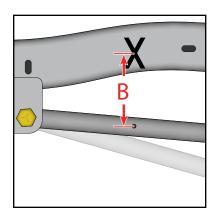
**Step 3.)** While standing clear, exhaust the vehicle to the very bottom of its travel. Now re-measure from your dot up to the center of your "X". We will call this distance "B".
