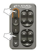
With the Ignition ON and the E-Brake ON, use the Manual Rocker Switches to *Raise/Lower* all four corners until each corner is at your preferred **MAXIMUM TRAVEL** and the vehicle is level from side to side.
