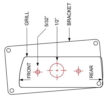
NOTE: The chamfered holes on the TouchPad bracket that attach the bracket to the grill must be facing up
