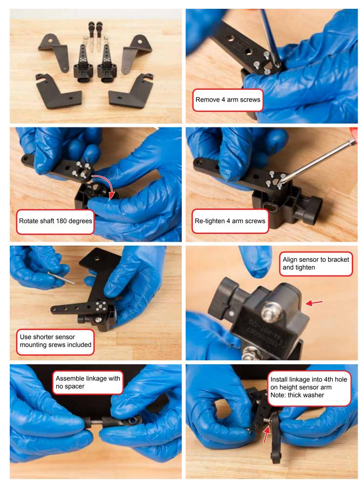
Audi B8 Rear Height Sensor Bracket Kit Assembly
