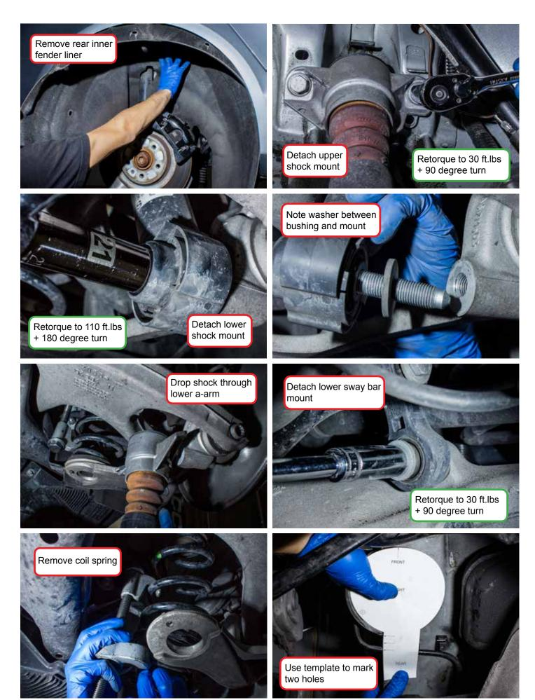
Audi B8 Rear Air Spring Kit Installation
