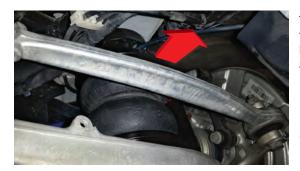
The curve of the toe link needs to be away from the air spring.
