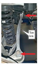
The toe link will be reinstalled opposite of the original orientation.
