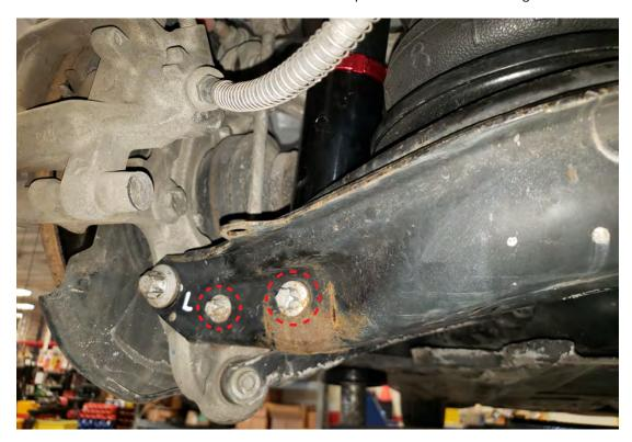
6. Secure the air spring assembly to the lower control arm with the centering spacer, lock washer, and bolt. Torque the bolt to 27Nm (20 lb.-ft.)
