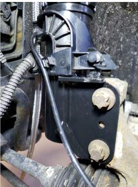
5. Attach the supplied end link to the damper and stabilizer bar. Torque to 98Nm (72 lb.-ft.).
