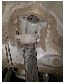
6. Disassemble the upper mount from the shock rod.
