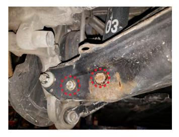
3. Support the lower control arm. Unbolt the lower control arm from the crossmember.
