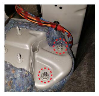
4. Insert the air spring assembly and nest into the lower control arm. Lift the control arm and attach to the crossmember. Do not torque until at desired ride height with load.
