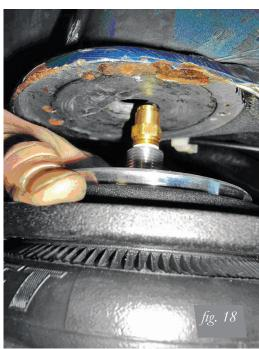
7. Thread the plastic nut onto the threaded boss (Fig. 19). If using 3/8" air line, install the fitting after the plastic nut is installed.
