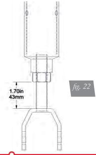
Your struts have been pre-set at the factory to provide maximum drop height while maintaining adequate tire clearance to the air spring. If you wish to gain more extended height (lift), which is the same as reducing drop height, or want to lower the chassis further and there is still adjustment available at the lower mount, please use the following procedure:
