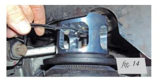
Apply the roll plate underneath the air spring. Lift the upper control arm and attach the air spring assembly to the control arm with the centering spacer (I), bolt (G) and lock washer (F) through the previously drilled hole. Torque to 20 Nm (15 lb.-ft.). (Figs. 15 & 16)
