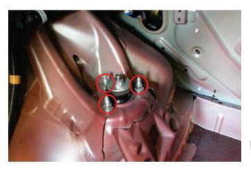
4. Remove the shock from the vehicle. (Fig. 8)
