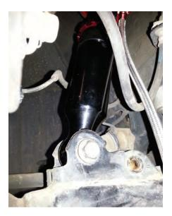
4. Reconnect the stabilizer bar link to the lower control arm (Fig. 16). Torque the nut to 84 Nm (62 lb.-ft.).
