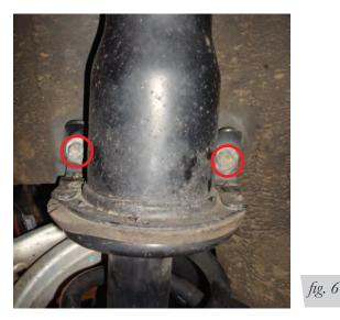
3. Within the luggage compartment, remove the trim and three upper shock mount nuts. (Fig. 7)
