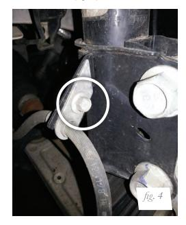
3. Unclip the sensor wire from the strut spindle tab. Unbolt and remove the two lower strut mount bolts (fig. 5).
