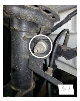
2. Unbolt the brake line from the strut (fig. 4).
