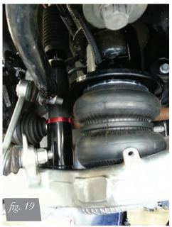
11. Route the air line in a manner that will not pinch or rub components and is away from heat sources.
