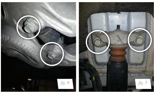
2. With the hub supported, unbolt the lower shock mount from the lower control arm (figs. 4 and 5).
