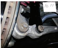
5. Align and attach the lower shock mount with the control arm (fig. 11). Torque to 88 Nm (65 ft-lbs.).
