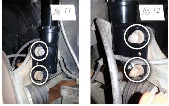
3. Reinstall the lower mount bolts through the strut mount connection (figs. 11 and 12).
