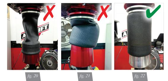
Caused by cycling with airline attached without pressure. Remove air-line from spring to release vacuum and re-attach. Inflate to 50+ PSI before lowering car to ground. Shows what spring looks like after lowering car to ground with <50psi and raising it with air pressure.
