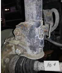
2. Unclip the sensor wire from the plastic clip. Remove the clip carefully from the strut, these can be brittle and could break easily. (Fig. 5)
