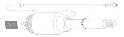
2. Fully seat the flexible adjuster extension on the damping adjuster and torque the set screw a half turn beyond hand tight. Remove the extension knob prior to vehicle installation. (Fig. 7)
