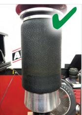
Shows what spring looks like when installed correctly.
