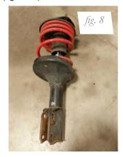
3. Unthread the three upper mount nuts and remove the strut from the vehicle (figs. 7 & 8).
