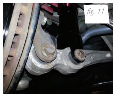
5. Align and attach the lower shock mount with the control arm (fig. 11). Torque to 88 Nm (65 ft-lbs.).
