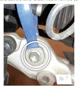
5. Disconnect the stabilizer end link from the lower control arm (Fig. 8).
