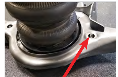
L-shaped feature is properly aligned in the hole
