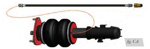
To gain full use of the camber plates, some inner fender modifications should be done
