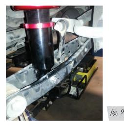
4. Raise the jack while guiding the upper mount into the holes in the chassis. Then thread the nuts on to the upper mount from inside the storage compartment and torque to 30Nm (22 lb.-ft.). (Figs. 10 & 11)
