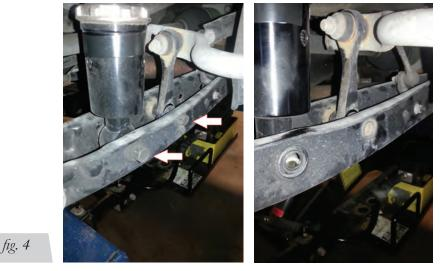
3. Remove the bolt for the lower shock mount and the sway bar end link to the lower
