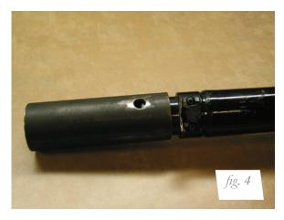
3. Slide the adapter tube back onto the strut body (fig. 4). Tack weld the adapter tube to the paint-free portions of the strut using the holes provided in the adapter (fig. 5).
