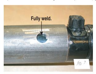
2. Fully weld the clevis to the adapter tube (fig. 8).
