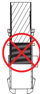
Not OK, threads are showing.
