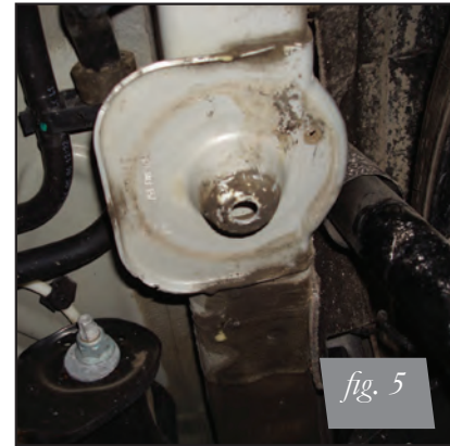
Previously Cut Spring Perch with Aftermarket Shock
