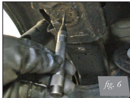
Previously Cut Spring Perch with Aftermarket Shock
