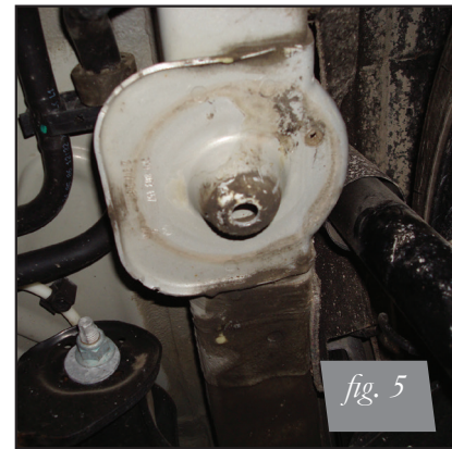
Previously Cut Spring Perch with Aftermarket Shock
