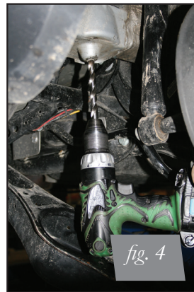
Previously Cut Spring Perch with Aftermarket Shock
