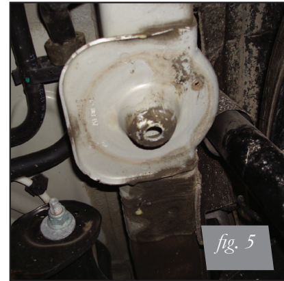
Previously Cut Spring Perch with Aftermarket Shock
