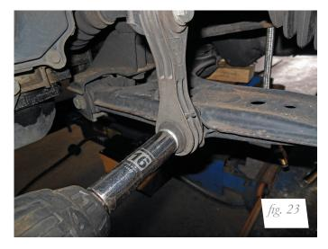
4. Reinstall the stabilizer end link to the control arm (Fig. 23). Torque to 30Nm (22 lb.-ft.).
