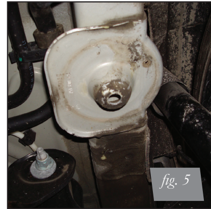
Previously Cut Spring Perch with Aftermarket Shock
