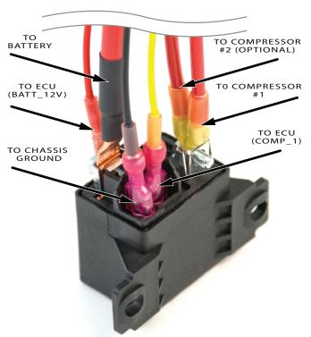
NOTE: AFTER CRIMPING, USE HEAT GUN TO SHRINK AND SEAL THE TERMINALS.
