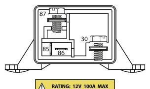
87 - TO BATTERY & TO ECU (BATT\_12V)
